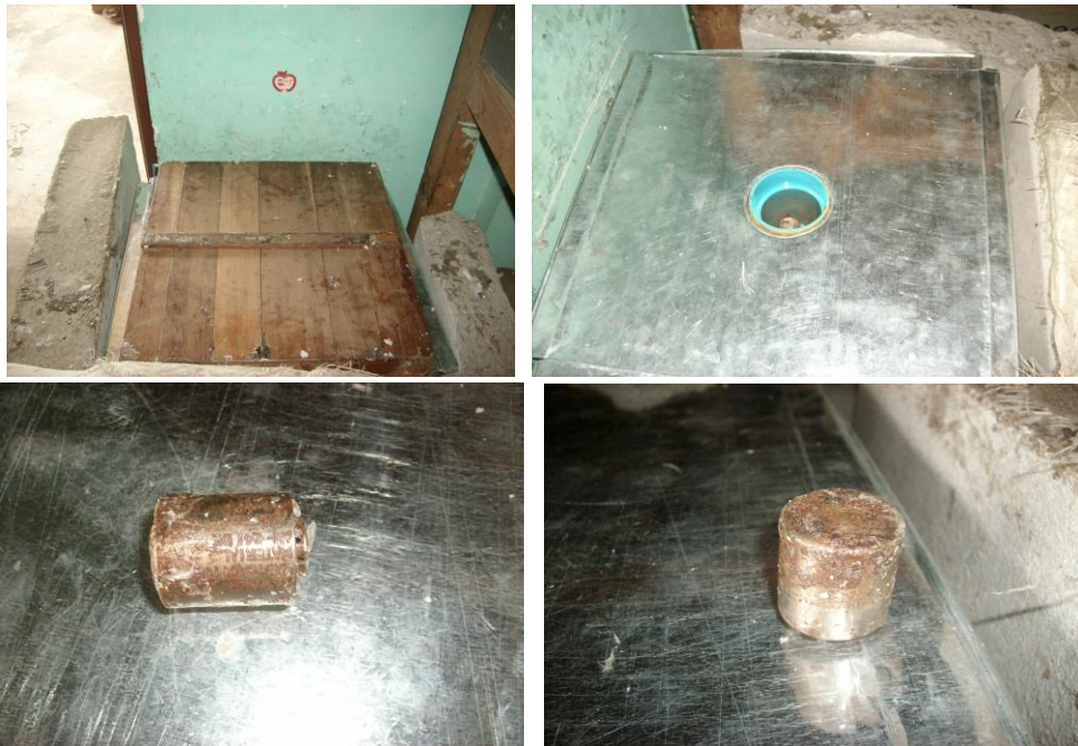
Figure 2: The experimental set-up of the 550mCi 241 Am-Be neutron source irradiation facility.
